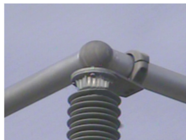
Corona in the base of the support, as expected from corona simulation.
